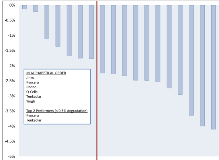
Figure 5-5 Humidity Freeze results
