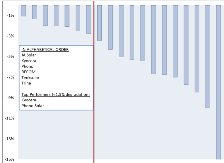
Figure 5-3 Thermal Cycling results
