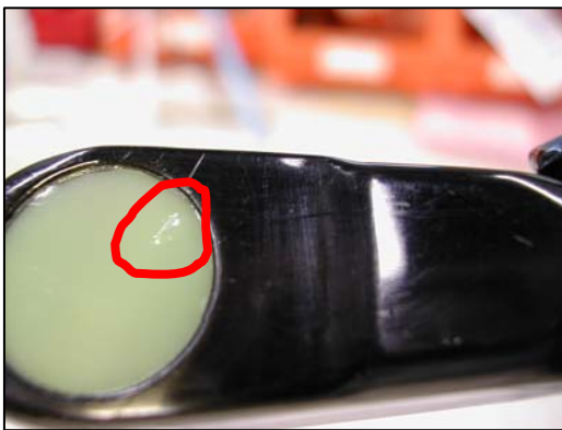
Scratching on the Lens
