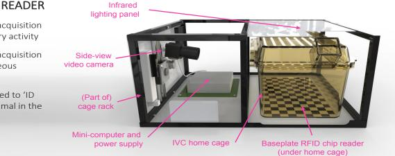
The camera is trained on the home cage enclosure 24 hours a day, and the baseplate reads data from the subcutaneously-inserted RFID chip in each rodent. This setup allows for each rodent's identity to be retained throughout every study. Infrared lighting ensures that no matter the time of day, data can be consistently collected.
