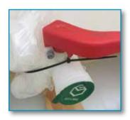
**Prior to discharge** a check of a tight and precise fit of the hose connection has to be done. It is recommended to secure the hose or pipeline close to the valve.
