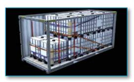
When fastening an IBC, appropriate straps and edge protectors have to be used to protect the IBC from damage, particularly, in the cage.
