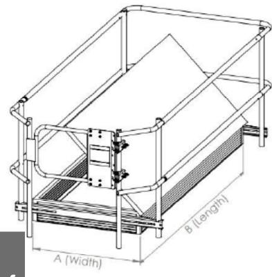
How to Measure: HatchProtector™ Roof Hatch Safety System
