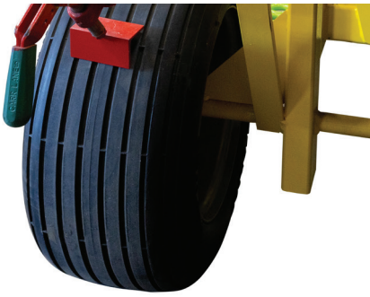
Wide flat free tires exert less pressure on the roof
