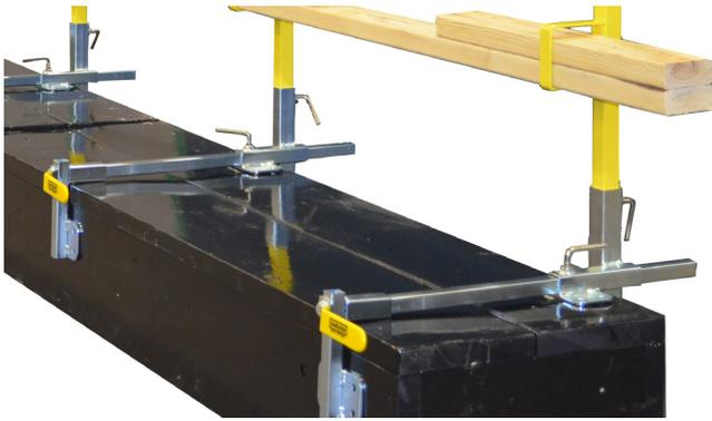
Typically the Perimeter clamp is clamped onto the vertical edge of a parapet wall. The stanchion is height adjustable to ensure the OSHA compliancy. Job site provided 2X4 lumber is used for the safety railing.
