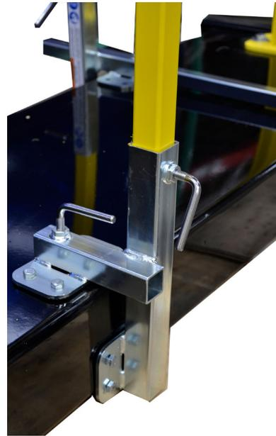
The perimeter clamp can be disassembled and mounted using four or eight 5/16" lag bolts driven into to a wood cap rather than the screw clamp method. This ensures no clamp protrusion into the roof top work zone which may inhibit certain types or work.
