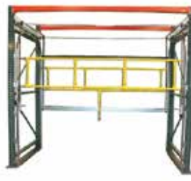
As inboard gate is opened, leading edge gate automatically closes.
