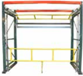
Gate closed on inboard side. Gate open on leading edge side. Place pallet into receiving area.
