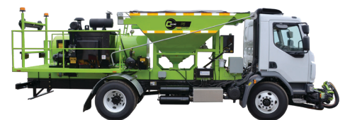
P5 One-Person Patcher with DuraPatcher Technology™
